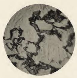
Fig. 14. Steel containing 0.45 per cent. C. Heated to 730° C. and quenched in water during critical range.
